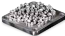
Partials, copings and bridges production in LaserForm CoCr (C)
